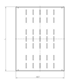
Material: SPCC Cold Rolled Steel; Thickness: 1.2mm
