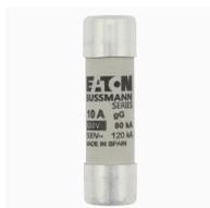
**Cartouche fusible, Basse tension, 10 A, AC 690 V, 80 kA, 14 x 51 mm, gL/gG, IEC**
