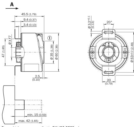
General tolerances according to DIN ISO 2768-mk  $\odot$  Cable diameter = 5.6 mm +/- 0.2 mm bend radius = 30 mm
