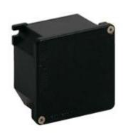
Distribution box for aggressive environments, AP series, external dimensions 100x100x59 mm / internal dimensions 88x88x44 mm
