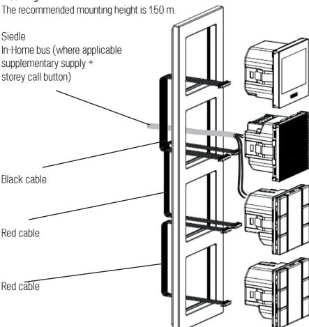
Each module is mounted in a flush-mounting junction box in compliance with DIN 49073. We recommend using a deep junction box for mounting. Mounting takes place using the provided supporting frames.
