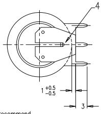
Note: 1)No welding onto the groove
