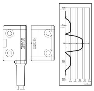
Assured switch on distance Sao 10 mm. Observe border areas for parallel approach: a minimum distance of 6 mm (typical) must be upheld when the actuator moves laterally to the sensor surface. This prevents early triggering due to the side preparation areas. "Standard" actuator, active side sensor surface
