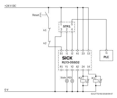
Parallel connection of two STR1 RFID safety switches to a Flexi Classic safety controller
