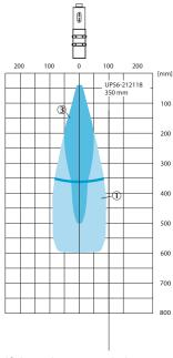
If the points named above are located in the radiation cone, reliable detection is guaranteed
