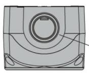
Knockout for M20/M25/PG13.5/PG16 (on top and bottom)
