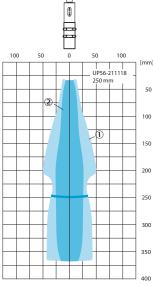
If the points named above are located in the radiation cone, reliable detection is guaranteed
