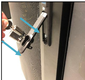
Step 4: Insert key and place tumbler in unlocked position. Insert tumbler into handle.
