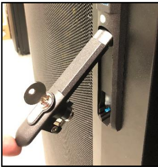
Step 1: Open handle with key in unlocked position.
