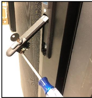
Step 2: Remove locking screw. Note: Do not discard the locking screw.
