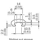
Sliding nut groove for side mounting
