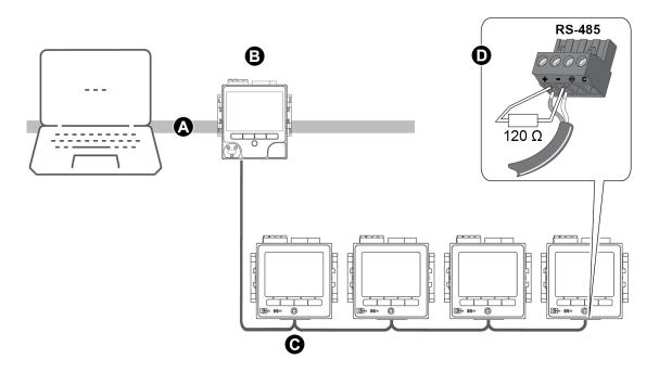
A LAN/WANB Ethernet gateway meterC Serial RS-485 network of devicesD Terminating resistor
