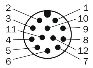
M12, 12-pin male connector, A-coded
