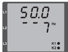
Fig. Screen for the mains frequency (50.0) and the direction of the rotating field.
