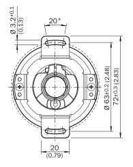
General tolerances according to DIN ISO 2768-mk (1) Cable diameter = 5.6 mm +/- 0.2 mm bend radius = 30 mm
