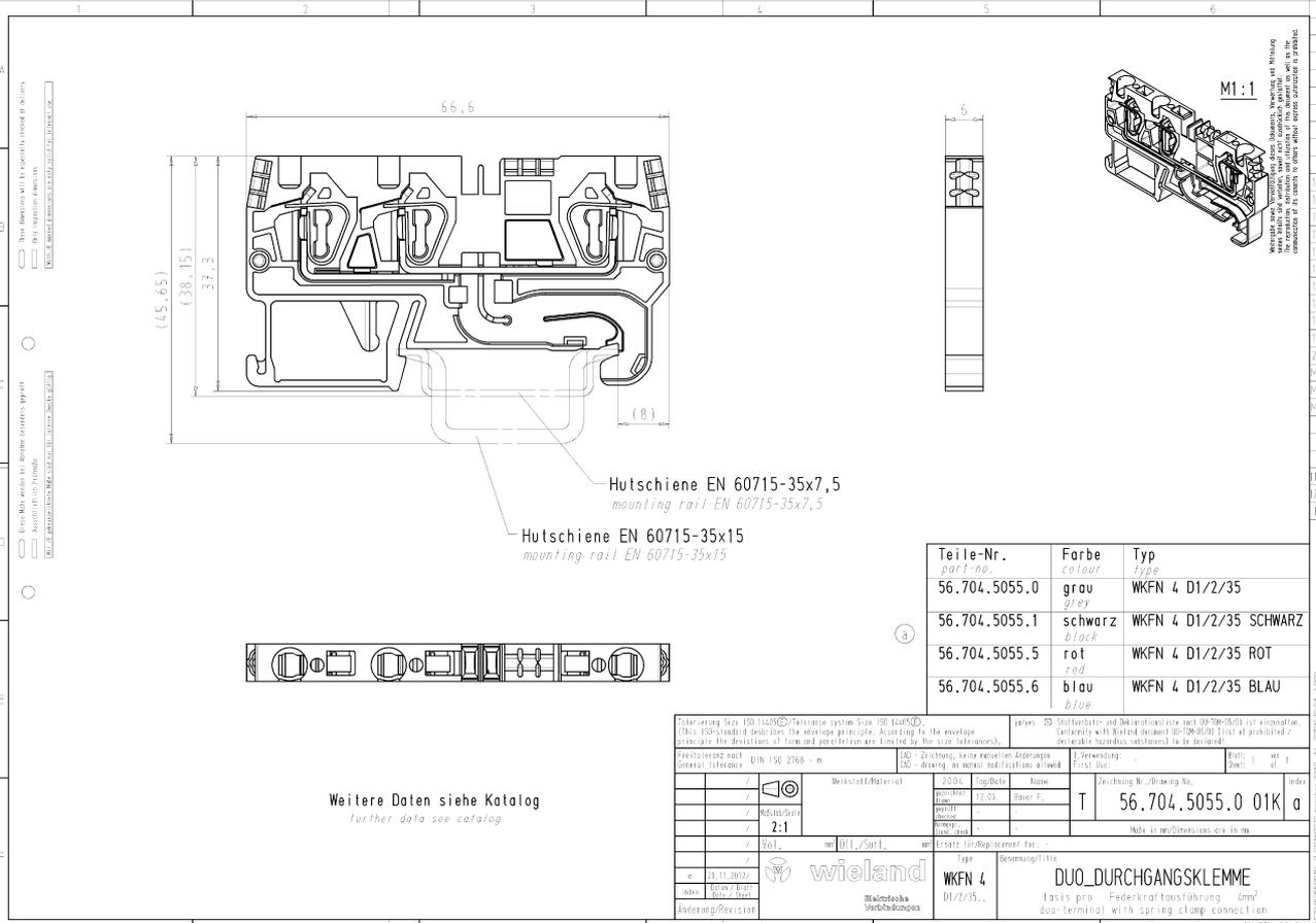
Technical drawing showing the front view, side view, and isometric view of a spring clamp terminal block. Dimensions include a width of 56.6 mm and a height of 37.3 mm. Callouts identify mounting rails: Hutschiene EN 60715-35x7,5 and Hutschiene EN 60715-35x15. A table lists part numbers and colors.
