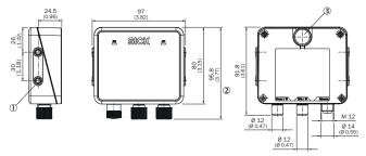
Structure and device dimensions, unit: mm (inch), decimal separator: period
