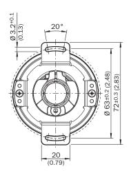
General tolerances according to DIN ISO 2768-mk ① Cable diameter = 5.6 mm +/- 0.2 mm bend radius = 30 mm
