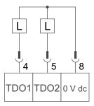
The following figure presents the sink wiring of the outputs. Sink or source can be configured on the digital output settings by the application.
