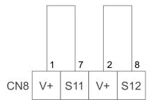
The following figure presents the wiring of an external emergency stop.
