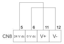
The following figure presents the wiring of the external power supply.
