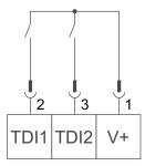
The following figure presents the source wiring of the controller digital inputs. Sink or source can be configured on the digital input settings by the application.
