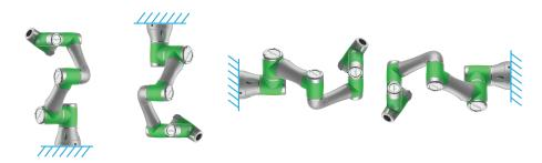
In case the Lexium Cobot Arm is mounted on a moving platform (for example, linear axis or moving platform), high acceleration of the moving ground base might be interpreted by the Lexium Cobot Arm as a collision.
