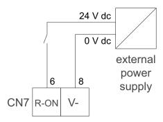
The following figure presents the wiring of the remote powering-off function at the Lexium Cobot Controller (CN7).
