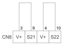
The following figure presents the default wiring of an external protective stop device.
