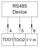
The following figure presents the wiring of the RS485 channel 2. RS485 communication can be configured on the analog input settings by the application.
