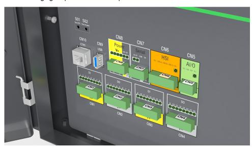
**NOTE:** Respective backgrounds of the terminals are marked by yellow (V+) and grey (V-) color. Terminals marked by V+ are connected to the internal 24 V dc power supply of the Lexium Cobot Controller, terminals V- are connected to the internal 0 V dc potential.
