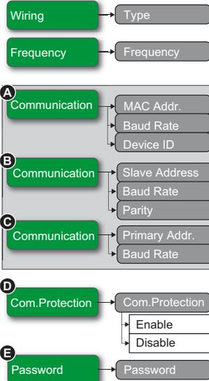
**en** Enter configuration mode and configure basic metering, communications, and security settings (see section 7 for instructions).
