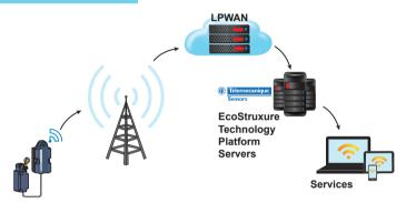
The XIOT11SE... standalone transmitter allows to exploit state changes from one to four dry contacts through a LPWAN connection (radio type). The transmitted information is made available on the web via a web browser or from IOS and Android mobile applications.
