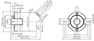
Non-tolerated dimensions according to DIN-ISO 2768-mk
