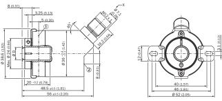
Non-tolerated dimensions according to DIN-ISO 2768-mk
