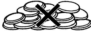
Example of stacked and jumbled batteries
