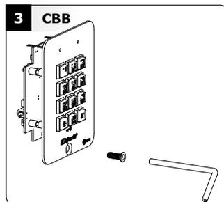
Take the flush casing to measure and mark the mounting holes. Then drill the 4 mounting holes and the wiring access area.
