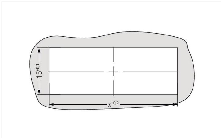
X = (pole no. x pin spacing) + 15.8 mm
