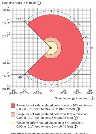
Attention! From the measurement origin up to a distance of 0.05 m (0.17 feet) no objects are detected (blind zone!) over the entire radial field of view (scanning range of  $270^{\circ}$ ). (6)
