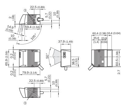
① Blind hole thread M5, 5 mm deep (2 x), for mounting
