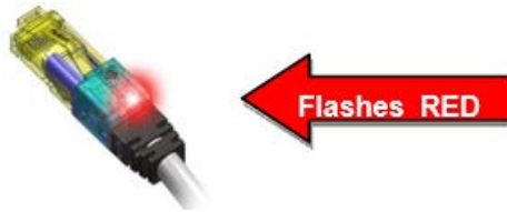
Figure 78: PViQ™ Enhanced I-Cord during a Guided Add (incorrect switch port connection)
