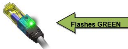
Figure 68: PVIQ™ Enhanced I-Cord during a Guided Add
