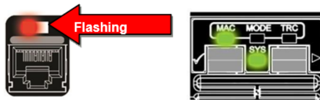
Figure 87: Designated Port and PViQ™ Panel IU during a Fiber I-Cord Authorized Remove
