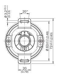
General tolerances according to DIN ISO 2768-mk ① Cable diameter = 5.6 mm +/- 0.2 mm bend radius = 30 mm
