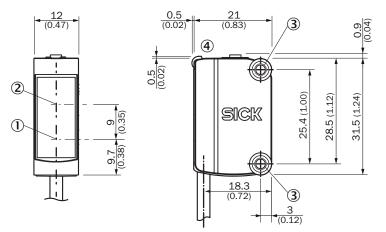
① Center of optical axis, sender
