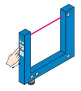
The yellow function indicator illuminates when the light received is at its optimum level. If necessary, increase sensitivity using the "+" button.
