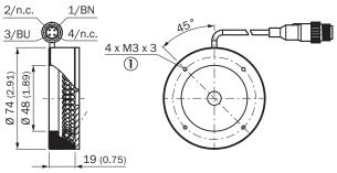
① For installation; pitch circle diameter 60 mm
