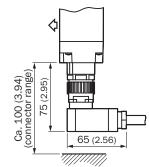
Cable sockets M26 x 11 + FE with crimp contacts
