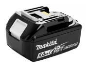
Li-Ion battery 18,0V 5,0Ah. Battery assembled with high energy cells to reduce the number of cells, pack dimension and overall weight. Built in shock absorbers for jobsite conditions. Battery fitted with a memory chip that communicates the usage history with the charger. Li-Ion technology without memory effect. Battery fitted with a cooling circuit for ultra-fast charge (Full charge 45 min using CLM1890-HC charger).
