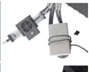
6 Close the sealing clip to ensure leaktightness.
