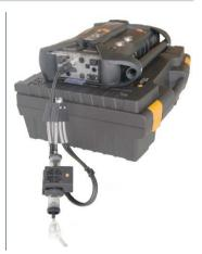
2 Connect the probe to the measurement gas inlet.
