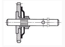
This device is situated inside the gearbox and is particularly recommended when gearbox protection is required in the event of accidental overloading.
