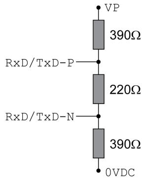
If the device is at the end of the network, use a Profibus connector with terminating resistor.
