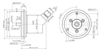
Order example for 6 mm shaft diameter: AHx36I-S3xx0xxxxx + BEF-FA-020-050-I (adapter is not pre-assembled)
