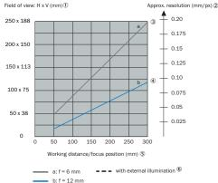
Take into account the following aspects when designing the application: the field of view geometry of the device, and the position of the field of view in the space in front of the device. Possible angles at which the objects can arise in relation to the device. For the planned working distance: resultant field of view length and width as well as the approximate resolution.
