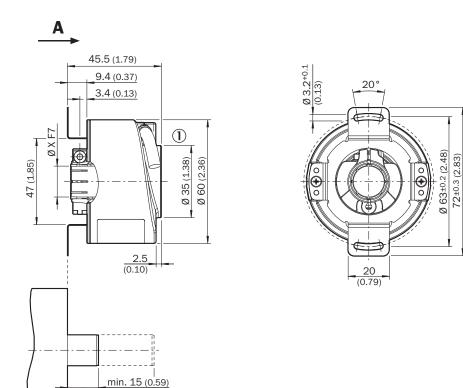
General tolerances according to DIN ISO 2768-mk (1) Cable diameter = 5.6 mm +/- 0.2 mm bend radius = 30 mm
