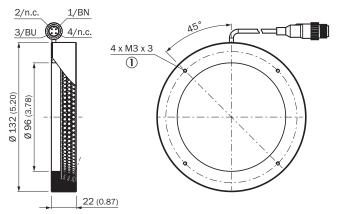
1 For installation; pitch circle diameter 116 mm
