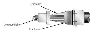
6. Pass the compound tube (3) over the conductors until the stepped end is fully located with the tube spacer (5). Pack more compound into place until the compound tube is fully filled.
