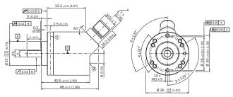
Non-tolerated dimensions according to DIN-ISO 2768-mk
