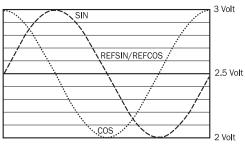
Signal diagram for clockwise rotation of the shaft looking in direction "A" (see dimensional drawing)1 period = 360 °: 1024
