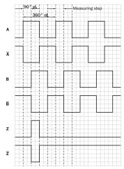
Cw with view on the encoder shaft in direction "A", compare dimensional drawing. ① Interfaces G, P, R only for channels A, B, Z.
