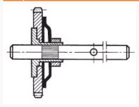
This device is situated inside the gearbox and is particularly recommended when gearbox protection is required in the event of accidental overloading.
