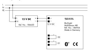
A voltage supply of 12 V DC must be connected on the input side.
