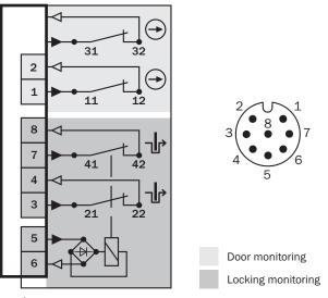
$\neg J_{\rm P}$  Positive action N/C locking monitoring contact  $\bigodot$  Positive action N/C door monitoring contact
